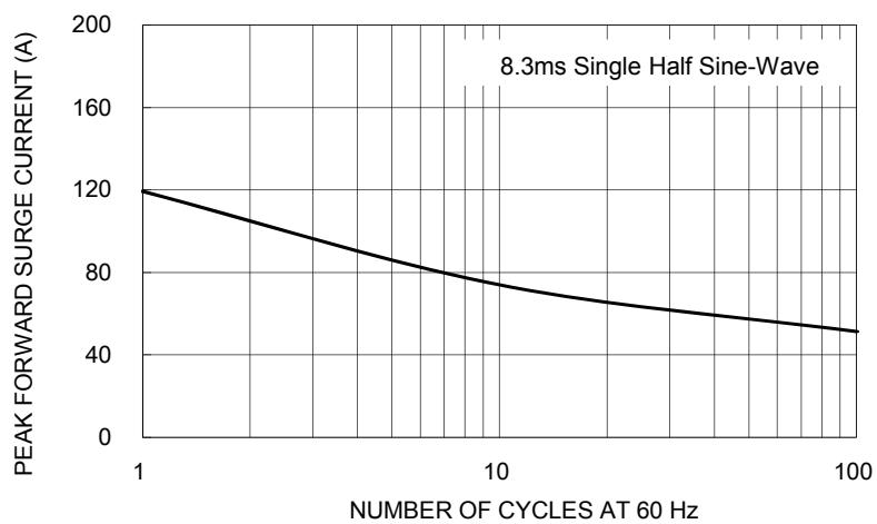
FIG. 3 MAXIMUM NON-REPETITIVE FORWARD SURGE CURRENT
